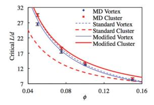
FIG. 4. (Color online) Critical length scale for vortex and cluster instabilities (i.e.,  $L_{Vortex}/d$  and  $L_{Cluster}/d$ , respectively) plotted as a function of solids fraction for e = 0.25. The solid and dashed lines correspond to the modified and standard theories, respectively.
