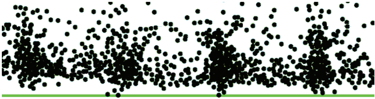
Figure 7. A snapshot of the MD simulation at the maximum opening of the gap ( t \approx 0.12 f^{-1} ), showing the material stuck at the bottom, between the peaks and the plate, whereas there is a completely empty space below the valleys.
