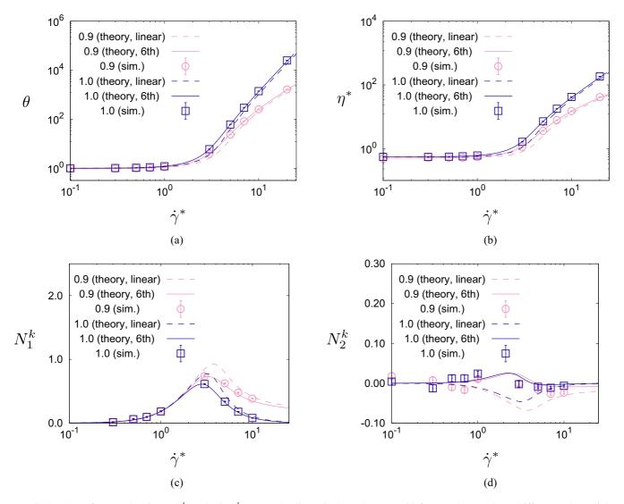
FIG. 4. Plots of (a)  $\theta$ , (b)  $\eta^*$ , (c)  $N_1^k$ , and (d)  $N_2^k$  versus the dimensionless shear rate  $\dot{\gamma}^*$  for  $\varphi = 0.10$  and two different values of the restitution coefficient: e = 1 and e = 0.9. The solid and dashed lines correspond to the (perturbative) theoretical results obtained in the sixth-order (denoted by "6th" in the legend) and first-order (denoted by "linear" in the legend), respectively. Symbols refer to computer simulation results.
