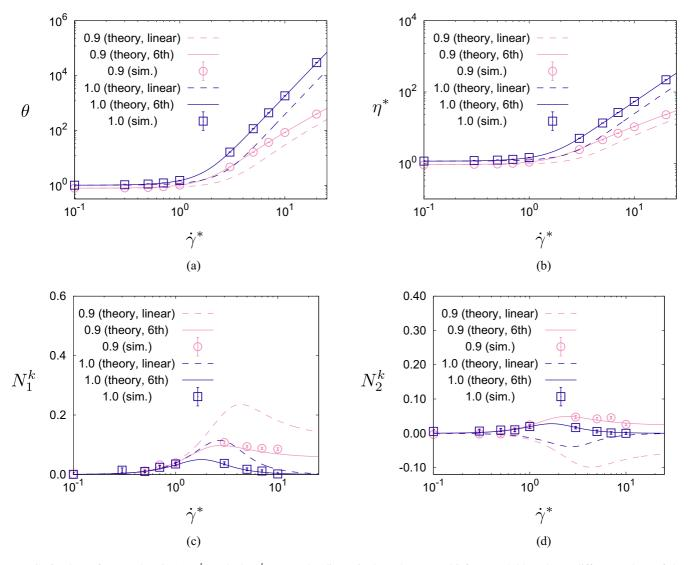
FIG. 6. Plots of (a)  $\theta$ , (b)  $\eta^*$ , (c)  $N_1^k$ , and (d)  $N_2^k$  versus the dimensionless shear rate  $\dot{\gamma}^*$  for  $\varphi = 0.30$  and two different values of the restitution coefficient: e = 1 and e = 0.9. The solid and dashed lines correspond to the (perturbative) theoretical results obtained in the sixth-order (denoted by "6th" in the legend) and first-order (denoted by "linear" in the legend), respectively. Symbols refer to computer simulation results.
