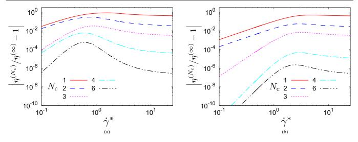
FIG. 1. Convergence of the shear viscosity against the truncation order in Eqs. (3.11) for  $\varphi = 0.30$  and e = 0.9. Two values of  $\xi_{ex}$  are considered: (a)  $\xi_{ex} = 0.1$  and (b)  $\xi_{ex} = 1.0$ . Here  $\eta^{(N_c)}$  represents the shear viscosity with the truncation to order  $N_c$ , while  $\eta^{(\infty)}$  is the nontruncated viscosity.
