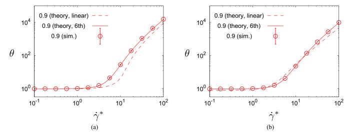
FIG. 9. Plots of the dimensionless temperature  $\theta$  against the shear rate for  $\varphi = 0.20$  and 0.30 (e = 0.9) when we consider the effect of the density dependence  $R(\varphi)$ . The dashed and solid lines represent the results from the linear approximation and arbitrary shear case truncated to sixth order, respectively.
