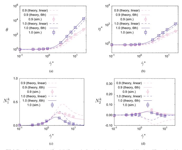
FIG. 5. Plots of (a)  $\theta$ , (b)  $\eta^*$ , (c)  $N_1^k$ , and (d)  $N_2^k$  versus the dimensionless shear rate  $\dot{\gamma}^*$  for  $\varphi = 0.20$  and two different values of the restitution coefficient: e = 1 and e = 0.9. The solid and dashed lines correspond to the (perturbative) theoretical results obtained in the sixth-order (denoted by "6th" in the legend) and first-order (denoted by "linear" in the legend), respectively. Symbols refer to computer simulation results.
