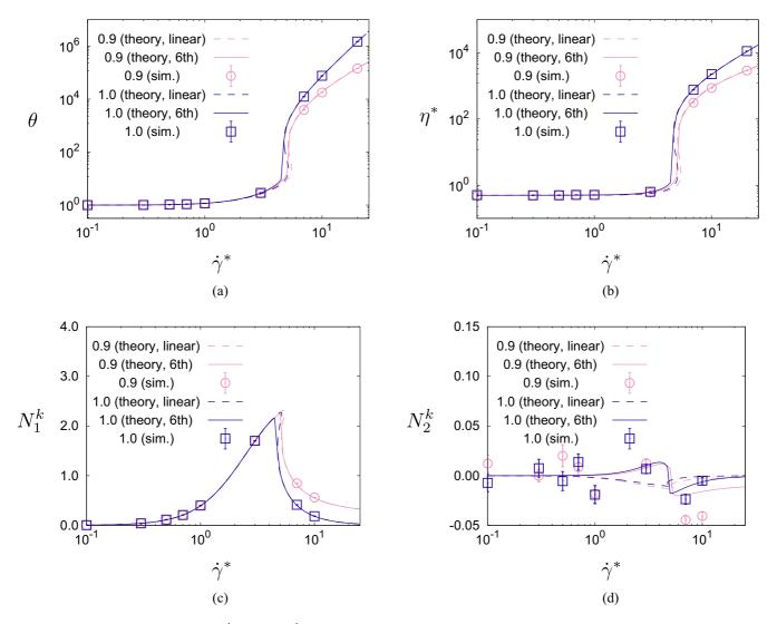
FIG. 2. Plots of (a)  $\theta$ , (b)  $\eta^*$ , (c)  $N_1^k$ , and (d)  $N_2^k$  versus the dimensionless shear rate  $\dot{\gamma}^*$  for  $\varphi = 0.01$  and two different values of the restitution coefficient: e = 1 and e = 0.9. The solid and dashed lines correspond to the (perturbative) theoretical results obtained in the sixth-order (denoted by "6th" in the legend) and first-order (denoted by "linear" in the legend), respectively. Symbols refer to computer simulation results.
