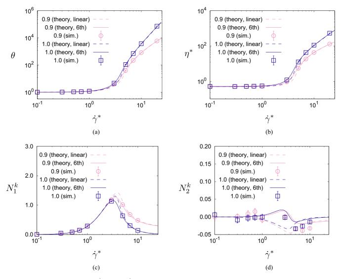
FIG. 3. Plots of (a)  $\theta$ , (b)  $\eta^*$ , (c)  $N_1^k$ , and (d)  $N_2^k$  versus the dimensionless shear rate  $\dot{\gamma}^*$  for  $\varphi = 0.05$  and two different values of the restitution coefficient: e = 1 and e = 0.9. The solid and dashed lines correspond to the (perturbative) theoretical results obtained in the sixth-order (denoted by "6th" in the legend) and first-order (denoted by "linear" in the legend), respectively. Symbols refer to computer simulation results.
