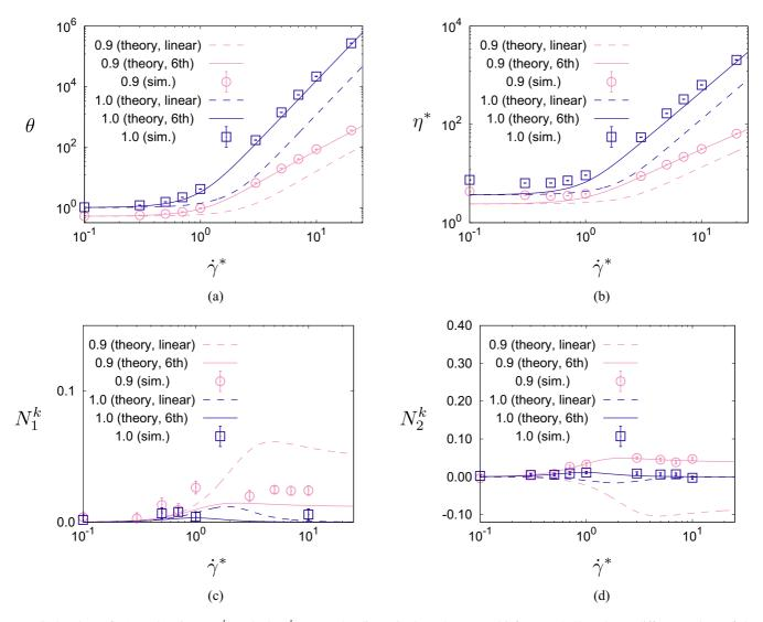
FIG. 8. Plots of (a)  $\theta$ , (b)  $\eta^*$ , (c)  $N_1^k$ , and (d)  $N_2^k$  versus the dimensionless shear rate  $\dot{\gamma}^*$  for  $\varphi = 0.50$  and two different values of the restitution coefficient: e = 1 and e = 0.9. The solid and dashed lines correspond to the (perturbative) theoretical results obtained in the sixth-order (denoted by "6th" in the legend) and first-order (denoted by "linear" in the legend), respectively. Symbols refer to computer simulation results.
