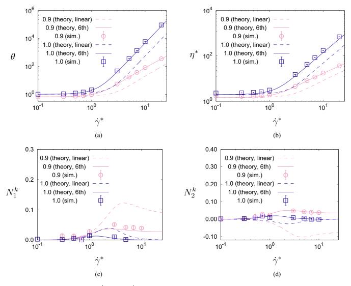
FIG. 7. Plots of (a)  $\theta$ , (b)  $\eta^*$ , (c)  $N_1^k$ , and (d)  $N_2^k$  versus the dimensionless shear rate  $\dot{\gamma}^*$  for  $\varphi = 0.40$  and two different values of the restitution coefficient: e = 1 and e = 0.9. The solid and dashed lines correspond to the (perturbative) theoretical results obtained in the sixth-order (denoted by "6th" in the legend) and first-order (denoted by "linear" in the legend), respectively. Symbols refer to computer simulation results.
