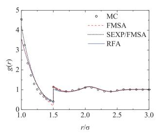
**Figure 5.** Radial distribution function g(r) as a function of distance r for an SS fluid having  $\lambda = 1.5$ ,  $T^* = 1$  and  $\eta = 0.4$  ( $\rho\sigma^3 = 0.764$ ) as obtained from the FMSA (dashed line), the SEXP/FMSA (dotted line), the RFA (solid line) and simulation data from Ref. [12] (circles).
