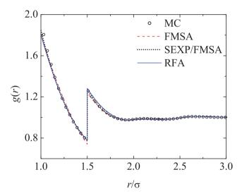
**Figure 6.** Radial distribution function g(r) as a function of distance r for an SS fluid having  $\lambda = 1.5$ ,  $T^* = 2$  and  $\eta = 0.2094$  ( $\rho\sigma^3 = 0.4$ ) as obtained from the FMSA (dashed line), the SEXP/FMSA (dotted line), the RFA (solid line) and simulation data from Ref. [21] (circles).
