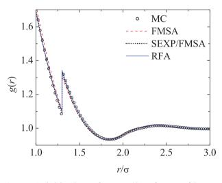
**Figure 2.** Radial distribution function g(r) as a function of distance r for an SS fluid having  $\lambda = 1.3$ ,  $T^* = 5$  and  $\eta = 0.2094$  ( $\rho\sigma^3 = 0.4$ ) as obtained from the FMSA (dashed line), the SEXP/FMSA (dotted line), the RFA (solid line) and simulation data from Ref. [21] (circles).
