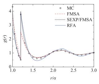
**Figure 1.** Radial distribution function g(r) as a function of distance r for an SS fluid having  $\lambda = 1.2$ ,  $T^* = 0.5$  and  $\eta = 0.4$  ( $\rho\sigma^3 = 0.764$ ) as obtained from the FMSA (dashed line), the SEXP/FMSA (dotted line), the RFA (solid line) and simulation data from Ref. [12] (circles).
