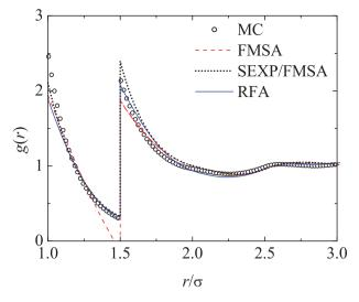
**Figure 3.** Radial distribution function g(r) as a function of distance r for an SS fluid having  $\lambda = 1.5$ ,  $T^* = 0.5$  and  $\eta = 0.2094$  ( $\rho\sigma^3 = 0.4$ ) as obtained from the FMSA (dashed line), the SEXP/FMSA (dotted line), the RFA (solid line) and simulation data from Ref. [19] (circles).
