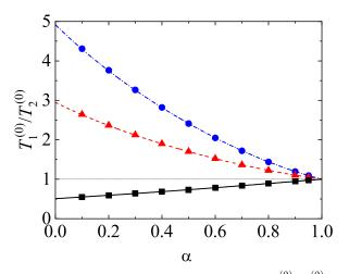
**Figure 5.** Dependence of the temperature ratio  $T_1^{(0)}/T_2^{(0)}$  on the coefficient of restitution  $\alpha$  for  $\sigma_1/\sigma_2 = 1$ ,  $x_1 = \frac{1}{2}$ ,  $\phi = 0$ , and three values of the mass ratio:  $m_1/m_2 = 5$  (solid line and squares),  $m_1/m_2 = 3$  (dashed line and triangles), and  $m_1/m_2 = 0.5$  (dash-dotted line and circles). The lines correspond to the theoretical results while symbols refer to the results obtained from the DSMC method.
