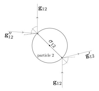
**Figure 2.** Direct and restituting inelastic binary collisions between two spheres of diameters  $\sigma_1$  and  $\sigma_2$ . The reflection law is  $(\hat{\sigma} \cdot \mathbf{g}'_{12}) = -\alpha_{12}(\hat{\sigma} \cdot \mathbf{g}_{12})$ . The coefficient of restitution satisfies  $0 < \alpha_{12} < 1$ . The dashed lines correspond to elastic collisions ( $\alpha_{12} = 1$ ). The action sphere around the particle of species 2 has the diameter  $\sigma_{12} = (\sigma_1 + \sigma_2)/2$ .
