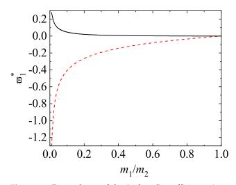
**Figure 14.** Dependence of the (reduced) coefficient  $\varpi_1^*$  versus the mass ratio  $m_1/m_2$  for a molecular binary mixture of hard disks (d = 2) when  $x_1 = \frac{1}{2}$ ,  $\phi = 0.25$  and  $\sigma_1/\sigma_2 = (m_1/m_2)^{1/2}$ . The solid and dashed lines correspond to the results obtained here and those reported by Jenkins and Mancini [47], respectively.
