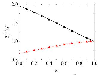
**Figure 8.** Plot of the temperature ratios  $T_1^{(0)}/T$  (solid line) and  $T_2^{(0)}/T$  (dashed line) versus the (common) coefficient of restitution  $\alpha$  for a dilute ( $\phi = 0$ ) ternary mixture (s = 3) with  $\sigma_1 = \sigma_2 = \sigma_3$ ,  $x_1 = x_2 = \frac{1}{3}$ ,  $m_1/m_3 = 5$ , and  $m_2/m_3 = 2$ . Symbols refer to the results obtained from the DSMC method (squares for the case  $m_1/m_3 = 5$  and triangles for the case  $m_2/m_3 = 2$ ).
