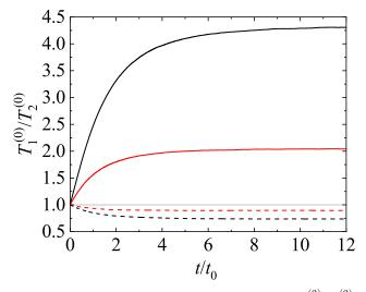
**Figure 3.** Time evolution of the temperature ratio  $T_1^{(0)}/T_2^{(0)}$  as obtained from the DSMC method for d = 3,  $\sigma_1/\sigma_2 = 1$ ,  $x_1 = \frac{1}{2}$ ,  $\phi = 0$ , and two values of the mass ratio:  $m_1/m_2 = 0.5$  (dashed lines) and  $m_1/m_2 = 10$  (solid lines). The black lines refer to  $\alpha_{ij} \equiv \alpha = 0.5$  while the red lines correspond to  $\alpha_{ij} \equiv \alpha = 0.8$ . Time is measured in units of  $t_0 = \ell_{11}/v_{th,1}(0)$ .
