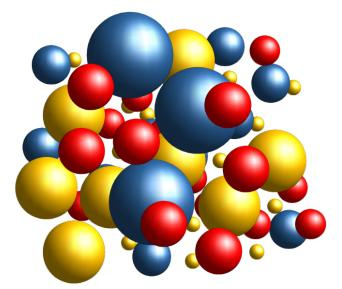
Figure 1. Schematic diagram of a ternary hard-sphere granular mixture.
