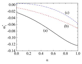
**Figure 15.** Dependence of the (reduced) coefficient  $\varpi_1^*$  versus the (common) coefficient of restitution  $\alpha$  for hard spheres (d = 3) with  $x_1 = \frac{1}{2}$ ,  $\phi = 0.25$ , and  $\sigma_1/\sigma_2 = (m_1/m_2)^{1/3}$ . Three different values of the mass ratio are considered:  $m_1/m_2 = 0.5$  (**a**),  $m_1/m_2 = 2$  (**b**), and  $m_1/m_2 = 5$  (**c**).
