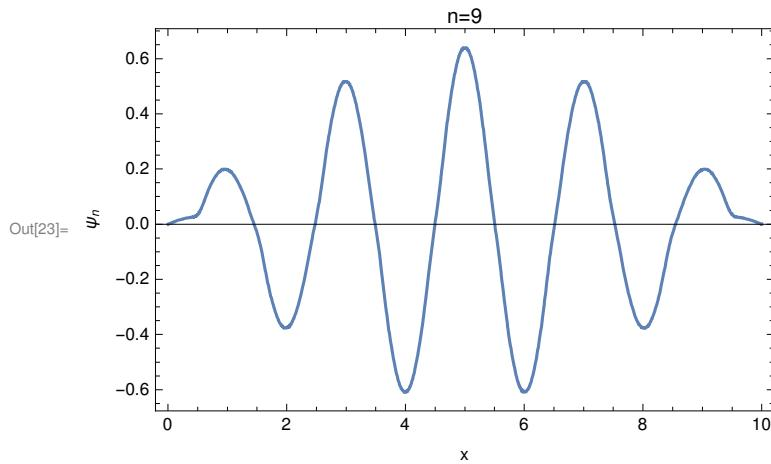
Eigenfunction  $\psi_n(x)$  with  $n=nLevel=10$  [see Fig. 3(c)]
